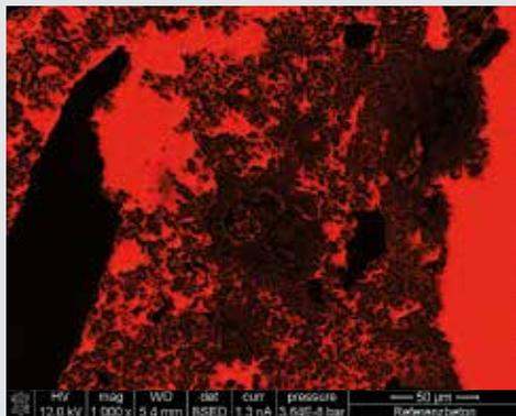
**Top: untreated concrete**, penetration of the resin indicates the original porosity of the cement paste that is relatable to the permeability of the paste.
