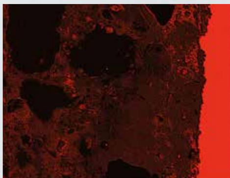
**Bottom: 2 layers of VANDEX SUPER crystalline slurry applied to cured concrete**
