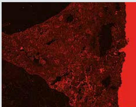
**Middle: VANDEX SUPER crystalline powder sprinkled into fresh concrete**
